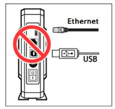
Do not connect USB cable and Ethernet cable at the same time.
